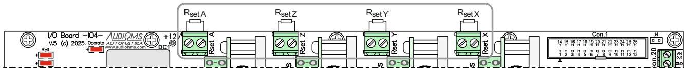
Figure 4.13 The position of the Rset resistor for adjusting the operating current of stepper motors
